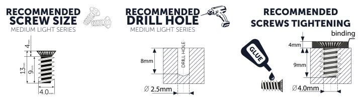
OGSO screw size recommendation is not obligatory. The screws coming with your binding will do the job just as well. Don't forget to apply glue to the screw before placing it in the drill hole. We recommend you choose a drill hole 1.5 mm smaller than the screw you select to ensure a tight fit.
